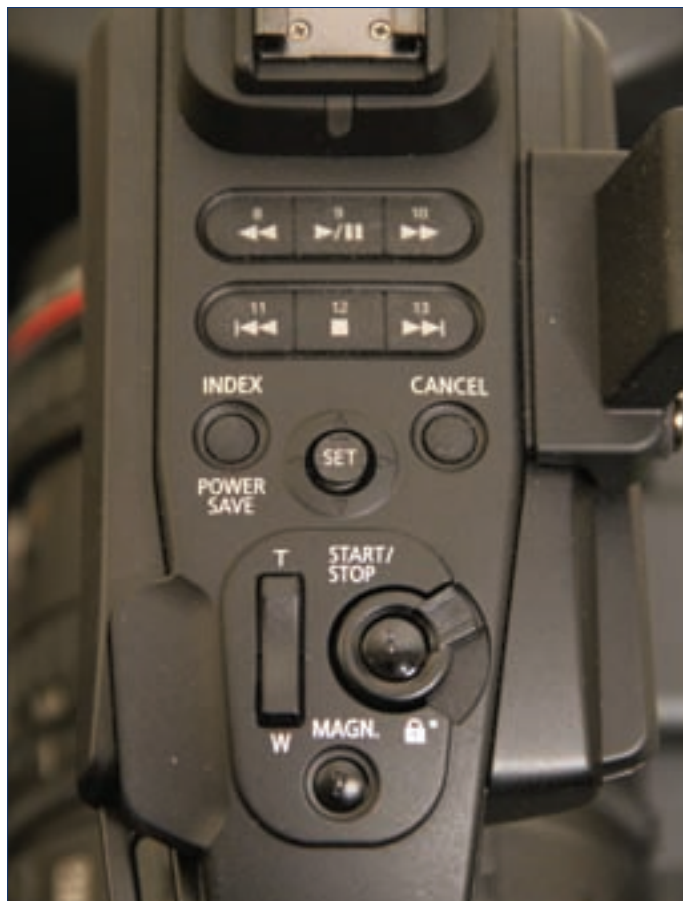
▼ The media playback buttons double up as assignable buttons in camera mode
